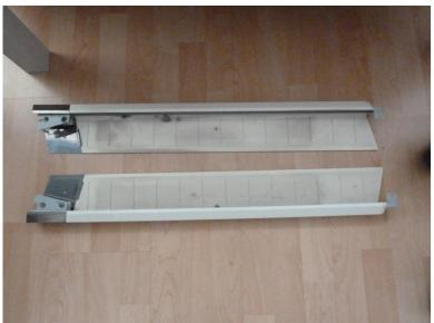
The reason for doing it this way around is there is a screw holding the front marquee trim in place and if you drop it - it goes all the way down the inside of these panels - by removing them you can put your hand under the end-plate and catch it if it falls out.
