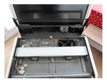
Disconnect cables for IO PCB and light (if fitted) that go through hole in right corner and tuck then into the base.
