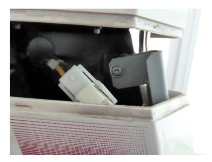
Remove the screw from the metal bracket and repeat for the other side. Remove the screw in the middle of the metal plates at control-panel height on side trim.
