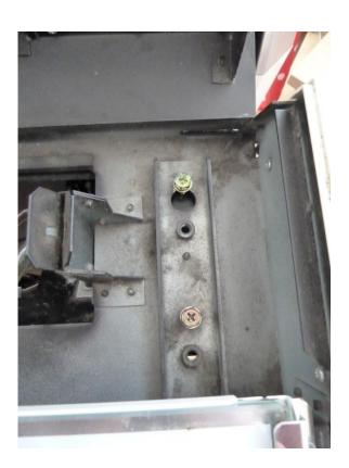
Remove the front one of each set and loosen the rear one - push the panel towards the screen slightly and you can lift the whole control panel assembly off.
