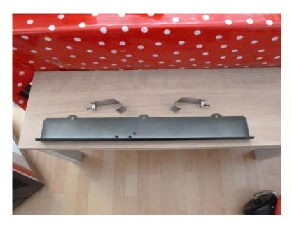
The plate covers the gap between the top of the cab and the top of the upper pair of speakers (as it's larger if screen is Yoko than when it's Tate).
