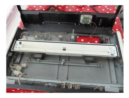
Remove the two screws at both ends on the light strip and it can be removed.
