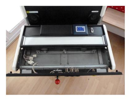
Remove the two large screws at the edges, hinge rear section open.
