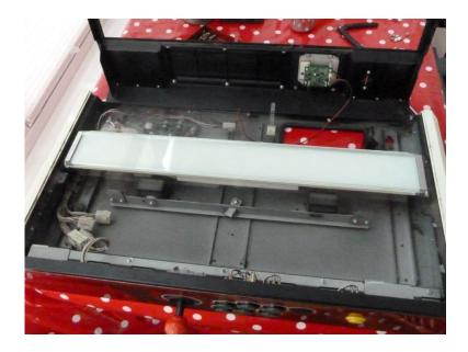
Remove 2 screws holding the metal glass-clips in place and remove from both ends, you can then remove the glass and diffuser.
