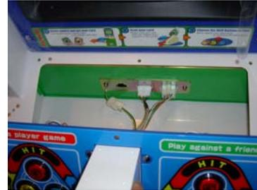
4. Remove the cord clamp and use nippers to cut the 2 tie belts loose.
