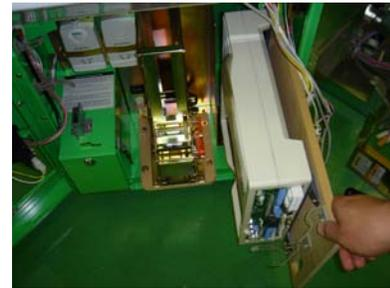
5. Remove the 4 screws and detach the NAOMI board from the base.
