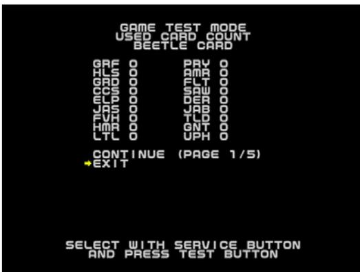
Select CONTINUE with the SERVICE Button and press the TEST Button to cycle through the pages (1/5, 2/5, ..., 5/5 and back to 1/5).
