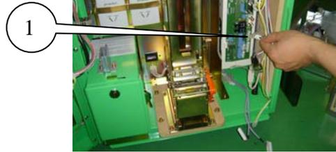
4. Remove the 1 wing bolt and pull out the ASSY MAIN BD.
