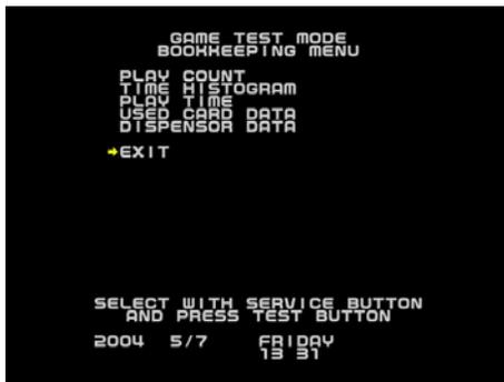
Use the SERVICE Button to move the cursor to the desired test item. Press the TEST Button to enter the selected item. After selecting an item, read the explanations below [(A) ~ (E)] regarding operation.
