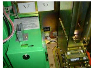
3. When it cannot be pulled forward any further, lift up on the card dispenser and detach it from the rail.
