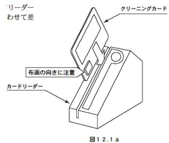
2. Slowly slide the Cleaning Card up and down to clean off any accumulated dirt.
