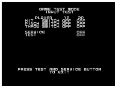
The input buttons are functioning correctly if each respective display changes from “OFF” to “ON” when pressing the input buttons.
