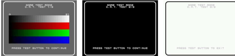
Pressing the TEST Button will display the “Color Bar”, “All Black”, and “All White” screens in order. Press the TEST Button again to return to the Game Test Menu screen.
