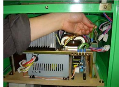
4. Remove the 2 wing bolts and pull out the board.
