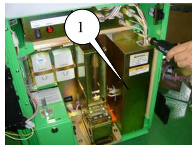
2. Loosen the 2 truss screws and detach the NAOMI cover.
