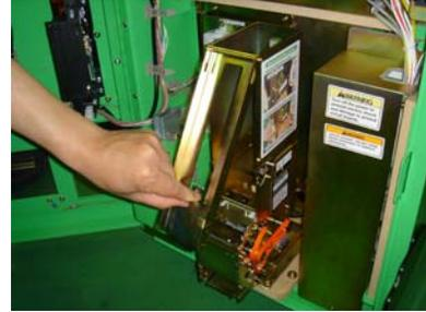
3. Take out the card weight. This part is covered in an air-wrap bag at the time of shipping.
