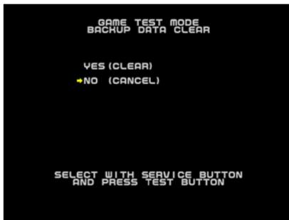
To clear data, use the SERVICE Button to move the cursor to YES (CLEAR) and then press the TEST Button.
