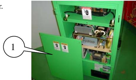
3. Unplug all the connectors plugged into the Power & I/O Board unit.
